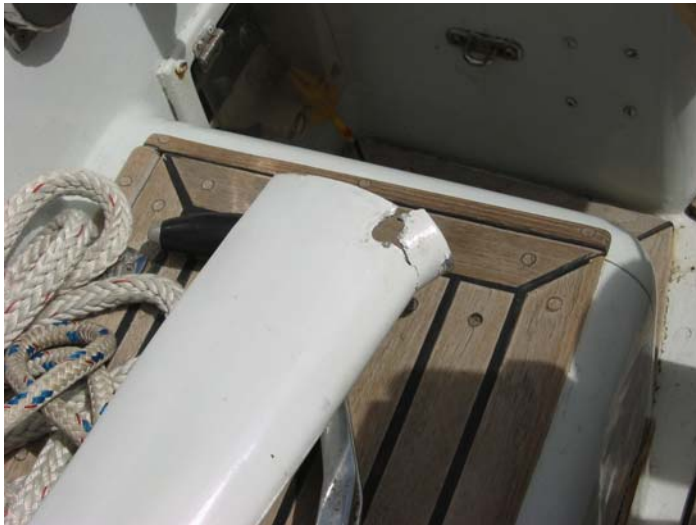
The broken spreader
