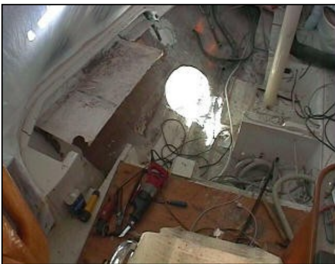
The circle that the piling scribed on the hull was used as a guide to open the hole The sole of our boat, the port settee, the forward head and the port fuel tank are gone.
