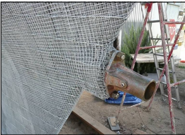
Port View: Cutlass bearing after a third layer of 1/2" mesh has been added over the 8 gauge wire.
