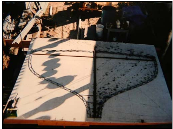
Framing Layout: The boat plans were transferred to the lofting platform at full scale. Each frame and the spine are then built to scale.
