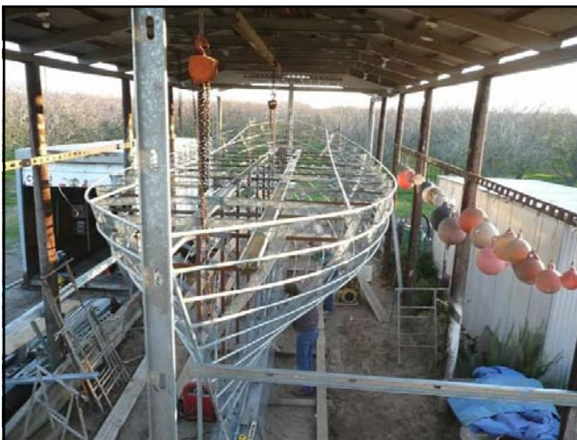
Forming: Pipe bent to meet the frames, forms the structure. This is a distinguishing feature of the Fred Lagier Ferro-cement System.
